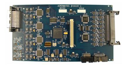
Model 682M is a mezzanine module for the PCIe-bus Model 1635AP Programmable Data Stream Processor telemetry system EU processing and data distribution card.
