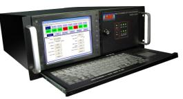
Control and monitoring of all parameters and features is accomplished by way of the local control interface using the built-in keyboard and touch-pad (**optional touch-screen**). Remote control of the unit is through an Ethernet interface. Remote Control Software is provided which mimics the local front panel on a remote PC.
