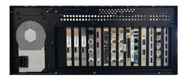
Configurable with HD-SDI Inputs, Acquisition Data, IRIG/GPS Time Code AM/AGC and Test Ports for Local ACU Option
