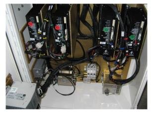
The Pedestal Interface | Init (PII I) contains all of the pedestal electronics
