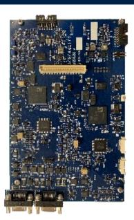
Incorporating a leading-edge FPGA, this modern design delivers a significantly reduced parts count, improved reliability, and expanded capabilities - including options normally found only in box level and multi-card bit sync/ encoder designs. The 674DM supports options such as Frame Sync Pattern Verification, BERT, PRN and programmable PCM simulator, and Convolutional encode/ decode.
