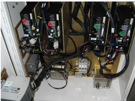
*The Pedestal Interface Unit (PIU) contains all of the pedestal electronics.*
