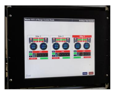
remaining systems on the network displayed along the side of the screen. This allows for control of an individual antenna while still monitoring the rest of the network. The MACU can monitor and control up to 8 ACU-M1s on an Ethernet based network.
